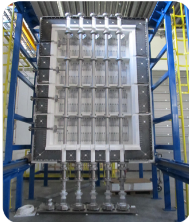
Fig. 1. Ultrasonic Spray Pyrolysis scale up equipment
